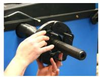
**Step 3:** Fasten the Cam Plate to the balancer hub using the supplied 5mm studs, washers and nuts.
