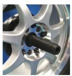
**Step 7:** Place the wheel onto the studs, in the same manner as you would when mounting the wheel on a vehicle. Use the 17mm lug nuts to hold the wheel. Tighten the lug nuts firmly, using a "star" pattern.
