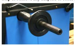
**Step 2:** Place the Cam Plate over the main shaft as shown. Align the mounting holes on the Cam Plate with the two holes on the balancer hub (arrows).
