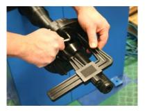
**Note:** If you are balancing a wheel that has a 3, 4, 6, or 8 lug pattern, it will be necessary to remove and reposition the cam arms into the correct holes on the Cam Plate. These holes are marked and can be easily identified. All other steps shown will remain the same.
