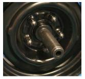
When the wheel is securely mounted, spin it by hand to make sure the wheel does not wobble. Balance the wheel following the instructions included with your wheel balancer.
