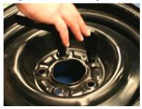
**Step 3:** Loosen the retaining screws on the Cam Plate. This will allow the cam arms to be adjusted to the correct bolt circle. Position the cam arms so that the stud spacing matches the caliper. When a cam arm is in the correct position, tighten the retaining screw on that cam arm. Repeat this step for all of the cam arms.
